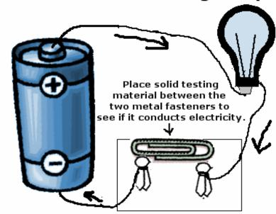
You can make a solid conductor testing set up with a battery, three wires, and a bulb as seen above. If a material is placed between the two metal fasteners that does conduct electricity, the bulb will light up. If the material placed between the fasteners does not conduct electricity, the bulb with not light up. In a way, by introducing a solid conductor into the circuit, and then removing it, you are creating a simple switch.
